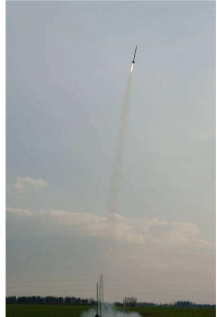
Martlet 0 reached almost 9,000ft and a maximum velocity of the speed of sound (760mph), with a motor with less than one third of the power that it was designed for. If Martlet 0 had been launched from a site with no altitude restrictions the flight would have reached around 14,000ft+ and 1400mph with a commercial 'L-class' rocket motor.
